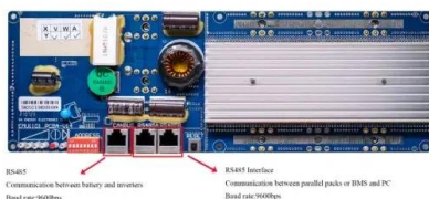
RS485 Communication between battery and inverter Baud rate: 9600bps RS485 Interface Communication between parallel grids or BMS and PC Baud rate: 9600bps
